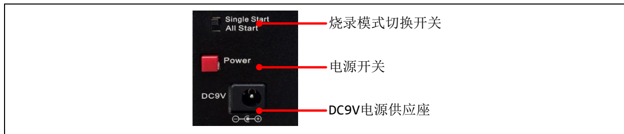
Figure 2-2 电源供应与烧录模式切换
